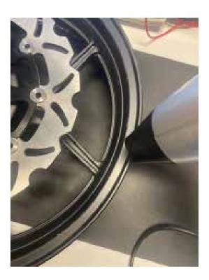
**2.** Apply the stickers little by little on the wheel rim, while heating the sticker slightly in order to make the glue set well on the rim.
