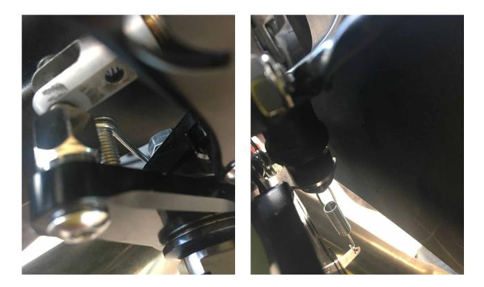
**5.** Install the pedal tip and the eccentric stop. Attach the heel protectors using the screws and small spacers provided with the kit,
