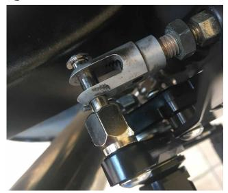
**4.** Install the brake pedal's "return" spring and the rear brake switch. (Use the spring provided for the brake switch, if needed, and adjust it to the right length for your motorcycle).
