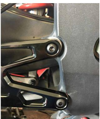
**3.** Attach the Master Cylinder to the rearsets' bracket using the allen screws and nuts and secure it to the brake pedal using the supplied axle and clip. When installing the brake pedal + footrest assembly, make sure the washer is properly positioned between the footrest bracket and the pedal with the rounded edge on the bearing side.
