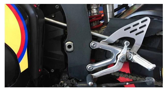
It is possible to set these rearsets in "reverse" (1st gear up) by turning at a 180° angle the connecting rod on the gear shift rod, but it will be necessary to shift the expansion tank.
