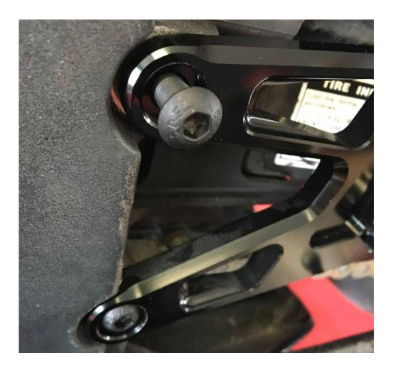
**3.** Install the gear shift pedal in the following order: Spacer > Gear shift pedal > Tapered / Conical washer > Footrest Position the spacer with the small edge on the gear shift pedal side.
