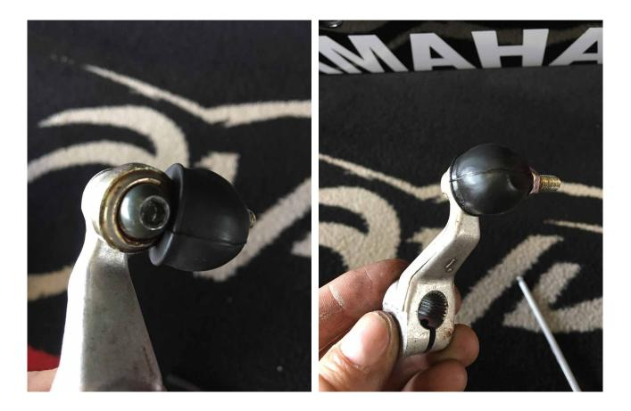
**5.** Reposition the gear shift rod and pedal so that the rod and pedal form an angle as close as possible to 90°.
