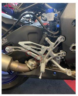
2. Unscrew the rear brake master cylinder fastening screws
