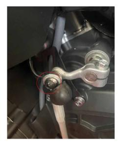
**2.** Fasten the intermediary bracket on the frame using the supplied screws and then fasten the main bracket on the intermediary one.
