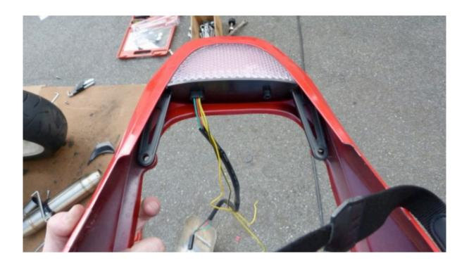
5/ To reinstall the rear fairing, you will need to make a small modification on your undertail (that's when the cutter comes to use).
