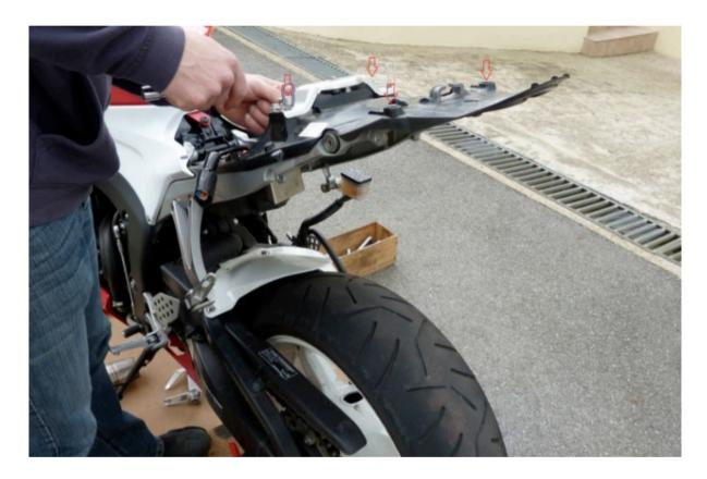
4/ Install the new tail light in the rear fairing you just uninstalled
