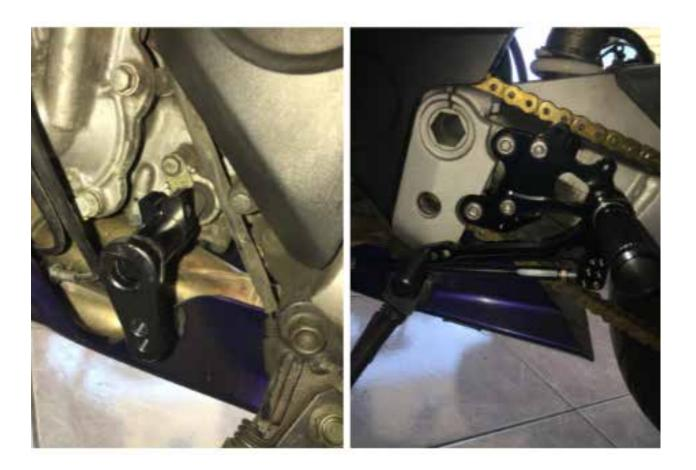
4. Attach the new ball joint to the gear shift rod (using the right screws and threads' direction), then fasten the ball joints to the gear shift lever and to the connecting rod support (for the rear ball joint, use the spacer).
