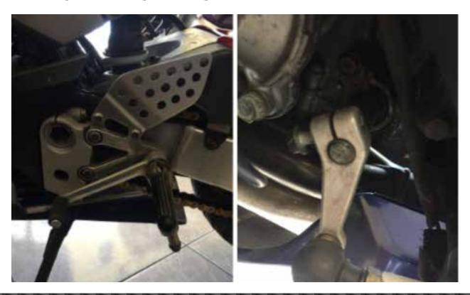
2. Assemble the footrest and the gear shift lever, and fix it to the foot rest bracket with the spacer (the washer's rounded edge must be facing towards the bearing, as well as the small edge of the spacer)
