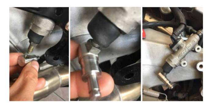
**4.** Assemble the foot rest with the pedal and the new bracket (Caution: the rounded side of the washers must be facing the bearing side).
