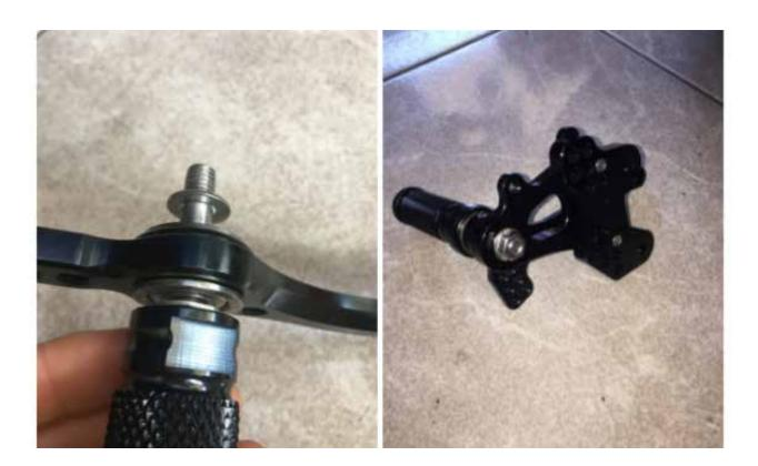
**5.** Attach the new foot rest bracket to the frame, using the original screws. Attach the MC and heel guard to the foot rest bracket using the screws provided with the rearsets. Then attach the Master Cylinder to the pedal using the washer and clip.
