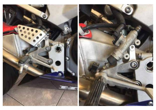
**2.** Unscrew the fixing screws of the original footrest bracket holding it to the frame and disconnect the brake switch from the foot-rests bracket.
