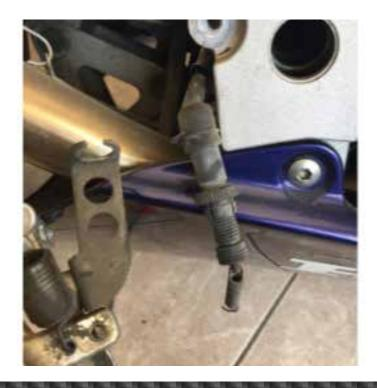
**3.** Screw the new MC junction piece to the new pedal. (Caution, the flat edge must be against the nut side)
