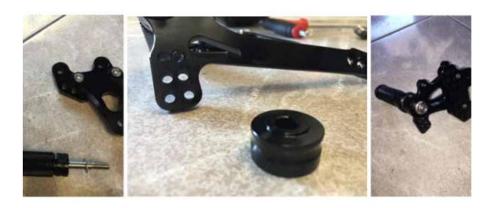
**3.** Install the new connecting rod's bracket to the gear shift axle. Then fix the new footrest bracket to the frame using the original screws.
