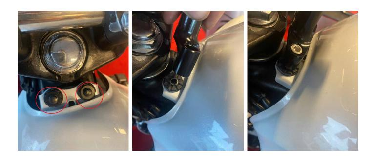
3. Install the steering damper's fastening clamp using the supplied M6 screw with round head and the 2 small washers with a 6mm diameter.
