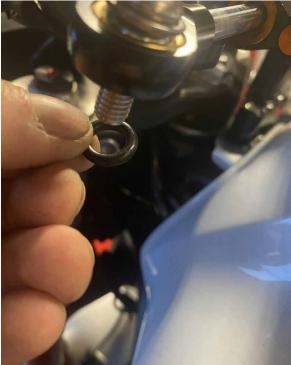
**5.** Adjust the hydraulic cylinder in the clamp before fastening it, in order to make sure that the steering damper, when turning left and right, does not come hitting against the tank.
