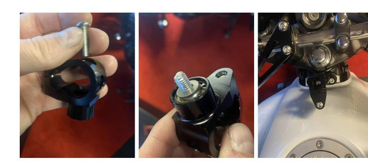
4. Insert the steering damper in the fastening clamp and fasten it to the triangle-shape bracket using the supplier M8 screw, the 8mm diameter washer and the 2 O-rings. Use 1 O-ring per side of the ball joint.
