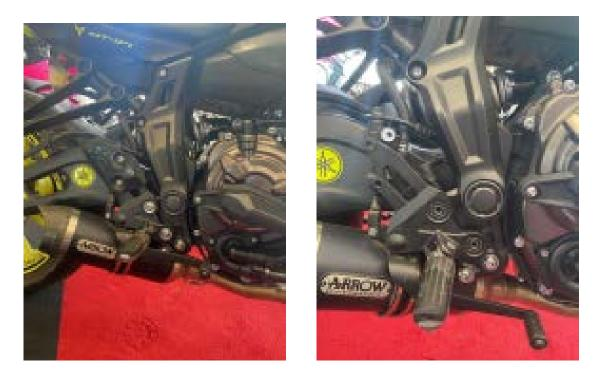
**2.** Disconnect the master cylinder from the brake pedal and disconnect the contactor
