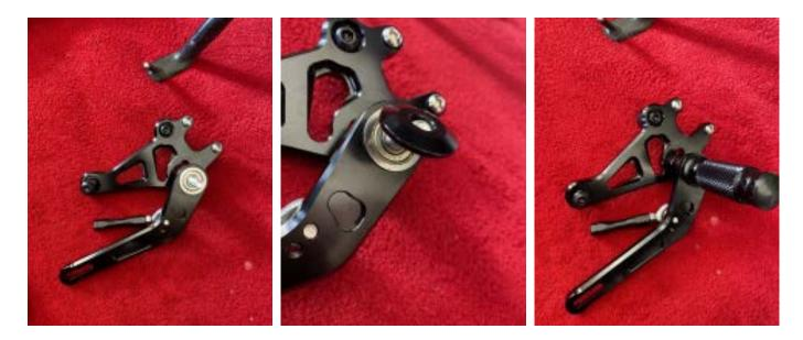
**3.** Attach the new bracket to the frame and screw the new rod onto the original one (Be sure to screw it them together correctly so that the rods do not come loose)
