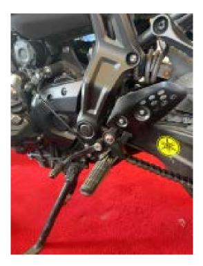
**2.** Assemble the new footpegs' bracket, making sure to position the large spacer behind the gear shift pedal, with the edge on the bearing side
