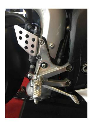
**4.** Install the new bracket with the supplied allen screws
