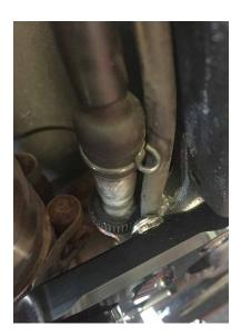
It is imperative to fix the brake fluid reservoir's hose to the brake hose coming from the MC with the nylon collar.
