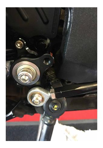
**4.** Attach the long rod with the supplied ball joints to the gear shift pedal and to the pivot, and fasten the short rod to the original pivot and ball joint remaining on the bike.
