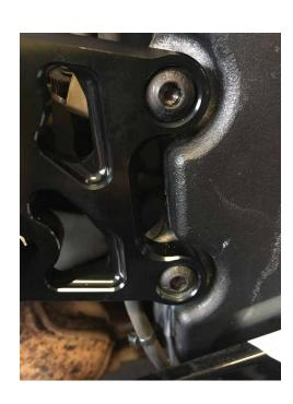
5. Reinstall the rear brake master cylinder with the supplied 2 allen screws for the upper part, and the axle and clip for the ball joint part (make sure to properly position the spring allowing the brake pedal to return). When installing the brake pedal, make sure that the washer between the bracket and the bearing is properly positioned, namely the rounded edge must be towards the bearing side.
