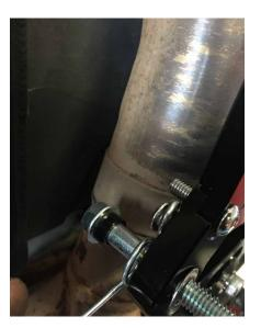
**6.** Install the footrest, and make sure to put the black conical spacer between the footrest and the bearing. Install the pedal tip and brake switch in their intended location.
