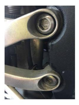
2. Disconnect the footrest bracket from the rear brake master cylinder (MC) by unscrewing the screw and nut holding the pedal to the MC (caution, there is a cotter pin), by unscrewing the 2 Allen screws holding the heel protector and the fixing screw of the aluminium guard (2 allen screws).
