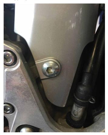
**3.** Disconnect the footrest bracket from the frame by unscrewing the 2 allen screws
