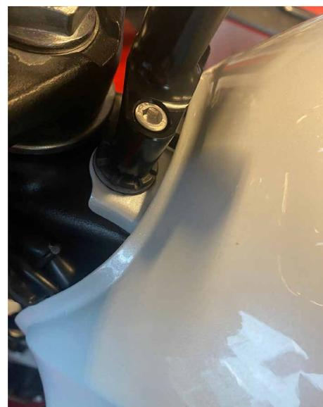
**3.** Install the steering damper's fastening clamp using the supplied M6 screw with round head and the 2 small washers with a 6mm diameter.
