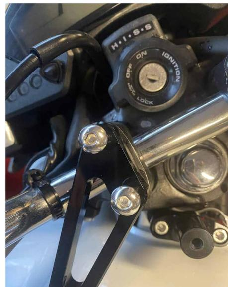
**2.** Take off the 2 screws fastening the front of your tank. Install the T-shape part using the supplied long M6 Hex screws (6mm diameter)
