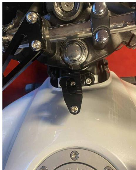
**4.** Insert the steering damper in the fastening clamp and fasten it to the triangle-shaped bracket using the supplier M8 screw, the 8mm diameter washer and the 2 O-rings. Use 1 O-ring per side of the ball joint.
