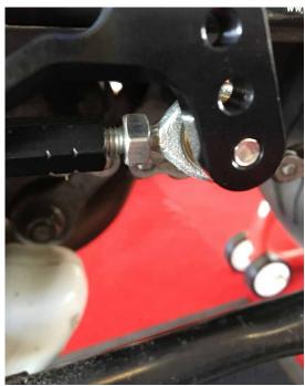
8. Install the heel protector using the small allen screws supplied with the rearsets
