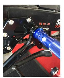
**5.** Fasten the gear shift lever's tip
