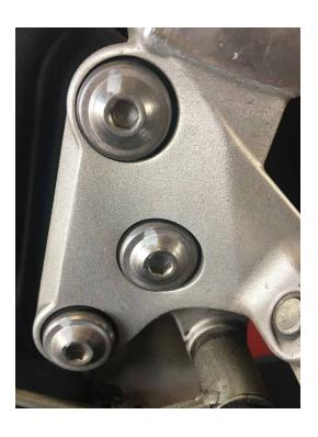
**3.** Install the rearsets' bracket using the supplied screws
