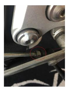
**2.** Unscrew the original bracket (3 allen screws)
