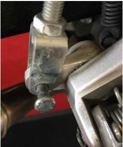
**2.** Uncouple the master cylinder from the original foot peg's bracket and dismantle the bracket from the frame
