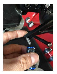
**6.** Screw the gear shift rod on the original ball joint, on the gear shaft side
