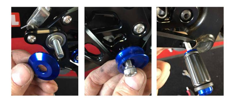
7. Install the heel protector and the brake switch spring, using the supplied screws and spacers (the brake switch spring is a universal part you will need to recut at the right length in order to install it)
