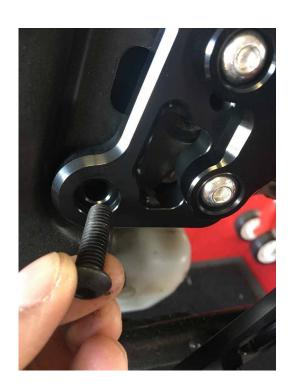
**4.** Install the Gear shift lever and Footpeg assembly (Caution, the black spacer will install with the small offset on the bearing's side)
