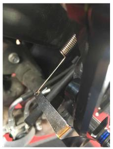
8. Attach the fluid reservoir using the supplied aluminium bracket, which you will need to shape according to the chosen location (in this case, the screw fixing the regulator bracket).
