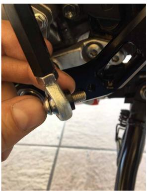
**5.** When adjusting the height of the gear shift lever, ensure that both ball joints are unscrewed approximately equally.
