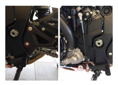
**2.** Fasten the rearsets' bracket with the supplied black screws.
