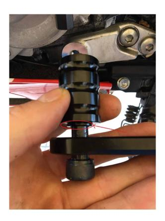
**4.** Screw the new ball joint into the rod. (Caution: use the model with inverted thread as shown on the picture). Attach the ball joint to the gear shift pedal using the screw and the small black spacer provided with the kit, between the ball joint and the gear shift.
