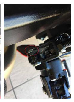
**2.** Attach the new pedal to the master cylinder using the new axle supplied with the rearsets, and using its screw and circlip. Insert the spring rod at the same time (see photo on the right).
