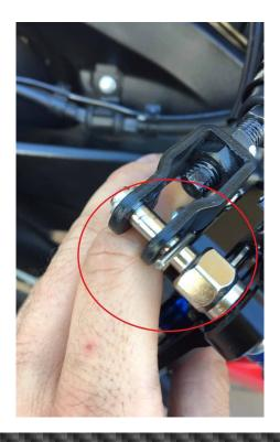
3. Re-install the master cylinder to the rearsets' bracket, the bracket to the frame, and the heel guard to the bracket with the supplied spacers.
