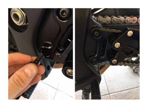
3. / Fix the new gear shift in place of the original one using the big BTR/Allen screw and the big spacer supplied with the kit (put the edge of the spacer on the bearing's side).
