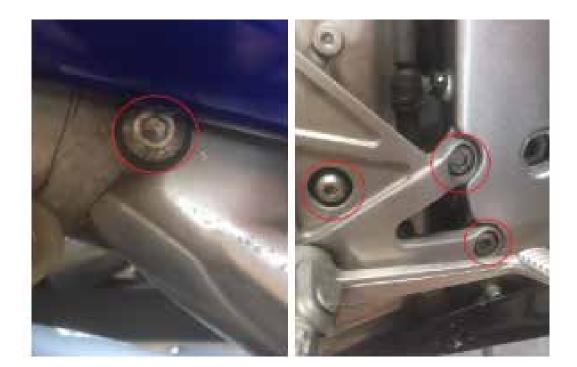
**3.** Installation of the adjustable rearsets' bracket on the frame (using the original screws) and of the footrest bracket using the screws supplied with the kit (Caution: the washers must be installed with the rounded edge towards the bearing).
