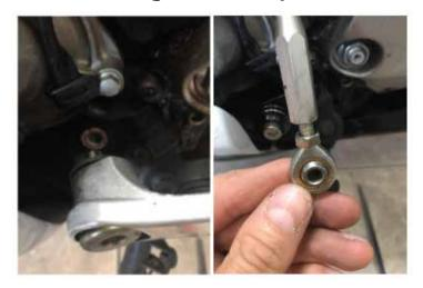
**2.** Fix the "pivot" part in place of the original gear shift lever (Small edge on the bearing side)
