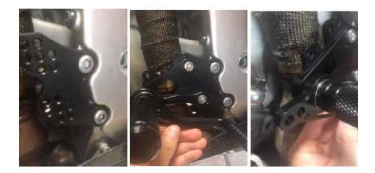
**4.** Re install the master cylinder using the screws provided with our rearsets. The pedal height is adjusted via the nut/counter nut on the ball joint of the master cylinder.
