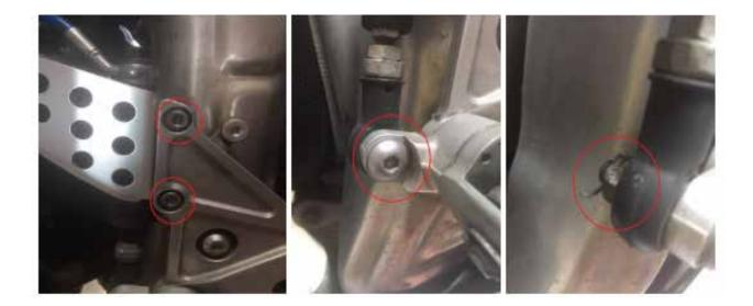
**2.** Remove the screws of the heat shield / heat protector and the screws holding the original bracket to your motorcycle's frame. We recommend you to put a new heat protector once the original bracket has been removed.
