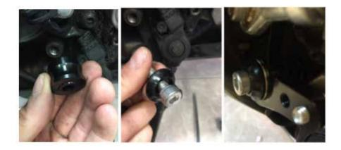
**3.** On the gear shift rod supplied with our rearsets, install the 2 remaining ball joints and fix this rod on the gear shift and on the "pivot" part (small ball joint on the gear shit side). Then fit the original rod on the "pivot" part
