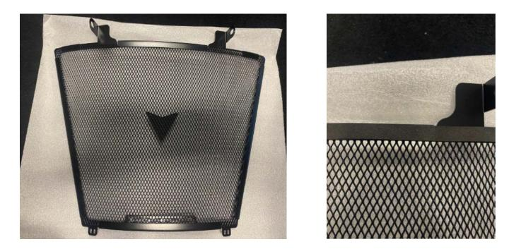
**2.** Unscrew the fastening screws from your radiator and install the grill over it using the original screws (depending on motorcycle models, screws can be placed differently)
