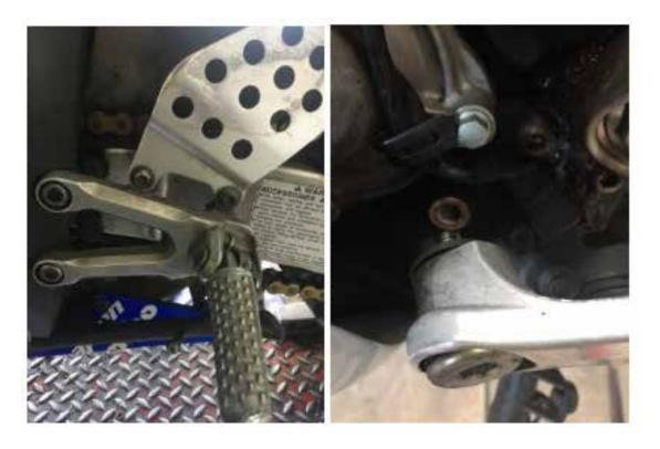
**2.** Re-install the new footpeg bracket with the original screws, and the heel protector with the screws supplied with our kit.
