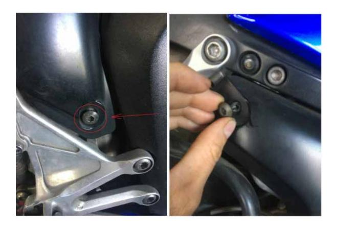
**2.** Remove the Master Cylinder mounting screws. And dismantle the original footrest bracket by unscrewing the screws fixing it to the frame.
