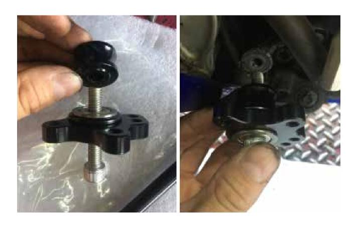
**4.** Attach the new ball joint to the original gear shift rod. Then on the pivot.
