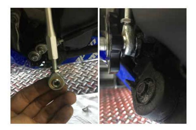
**5.** Attach the supplied connecting rod to the pivot and the gear shift lever. (caution, on the gear shift side, remember to put the small spacer between the ball joint and the gear shift lever)
