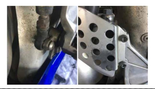
3. Attach the small bracket from the rear using the screws provided with our kit. Then fix the main bracket on the frame using the original screws of your footrest bracket.
