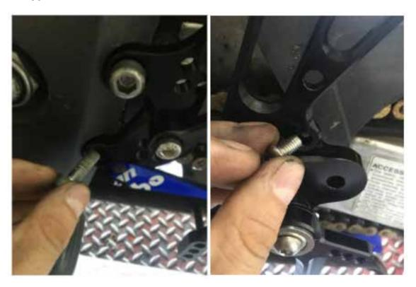
**3.** Install the pivot piece with the supplied spacer (Caution, the edge of the spacer must be on the bearing side)
