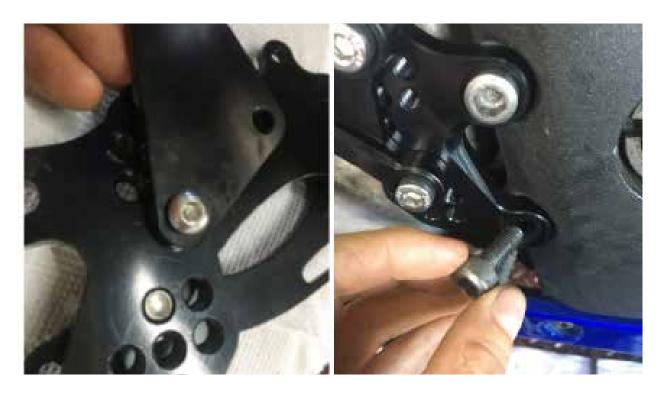
**4.** Install the supplied spacer in the Master Cylinder ball joint (Caution : with time, oxidation may form in the eyelet and make the installation of the spacer a little difficult). Attach the MC to the brake pedal and to the foot rest bracket using the screws provided with our rearsets.
